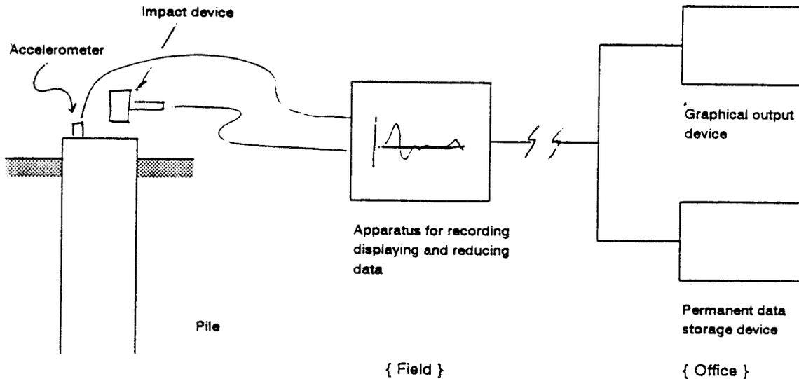
FIG. 2 Schematic Diagram of Apparatus for Integrity Testing
