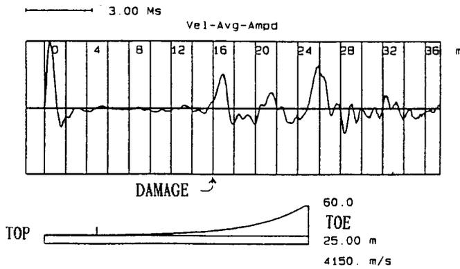
**FIG. 4 Typical Velocity Record Indicating Major Changes in Impedance (Severe Damage or a Cracked Pile (note the orientation of the input pulse is shown as positive in this standard; orientation could also be shown negative) )**
